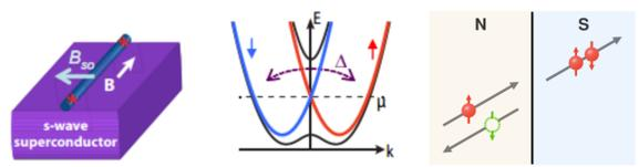
(a) Conceptual MF device.<sup>1</sup> (b) Energy dispersion diagram for a 1D semiconducting wire with Rashba spin orbit interaction (SOI). Magnetic field induces a Zeeman gap at  $k=0$  and superconductivity induces a gap  $\Delta$ .<sup>1</sup> (c) Schematic of Andreev reflection at a superconductor-semiconductor interface, an effect used to estimate  $\Delta^*$ .
