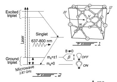
Vectorial magnetometry based on photon-induced Zeeman shift in energy levels of NV centers in a diamond lattice
