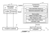
(57) Abstract: The vectorial magnetometer association of the detected spin-state-altering energy level and the corresponding defect orientations can be performed by generating Rabi flopping at each one of the energy levels and performing the association based on the detected Rabi flopping.
